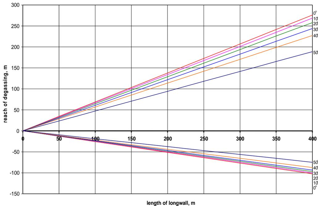
Fig. 1. Dependence of the degassing reach of undermined and overmined seams on the and slope of the longwall
