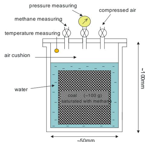
Fig. 5. Autoclave used in the tests
