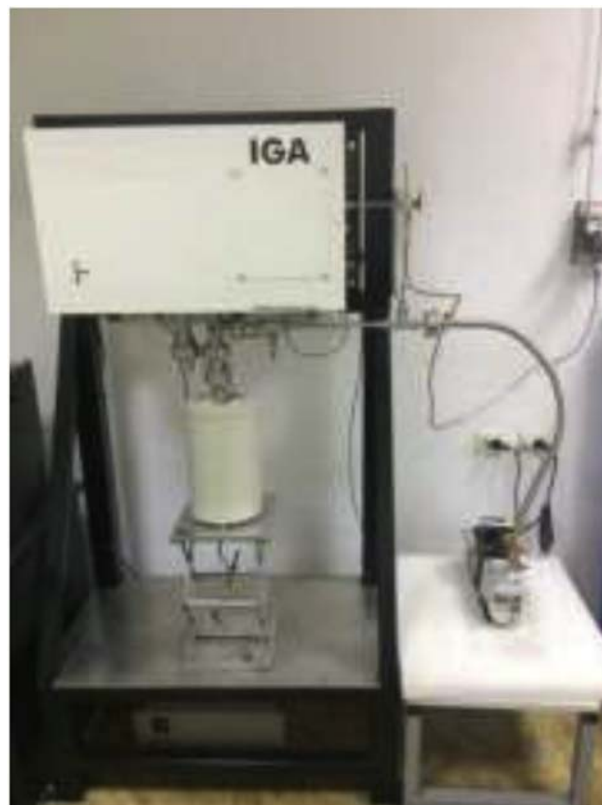
Fig.1. Gravimetric analyser IGA-001 to test gas sorption.
