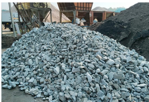
Fig. 3. Test sample of Greywacke (pic. Krzysztof Kurus).
