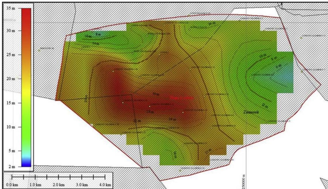
Fig. 6. Isoline coal-bearing potential map of Łędziny deposit.
