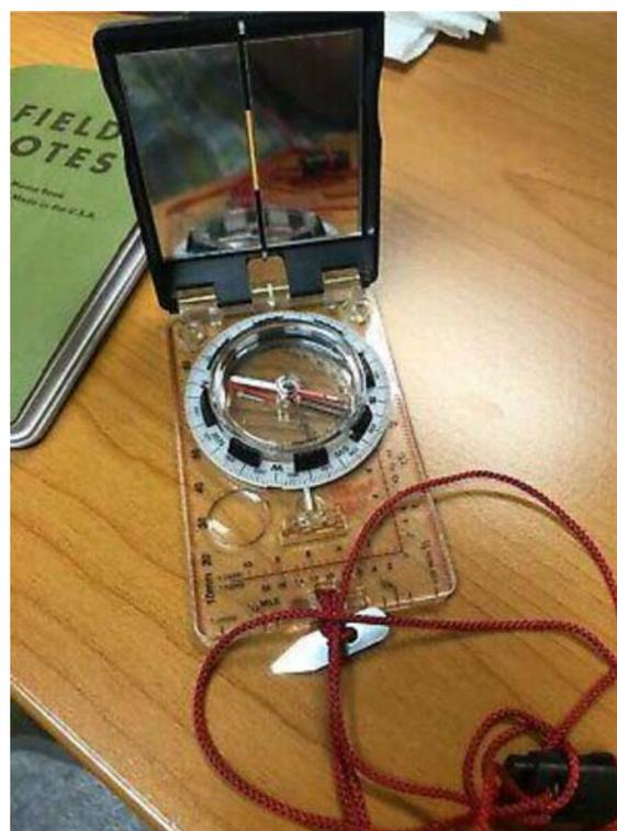
Fig. 4. Image of Silva foldable geological compass.
