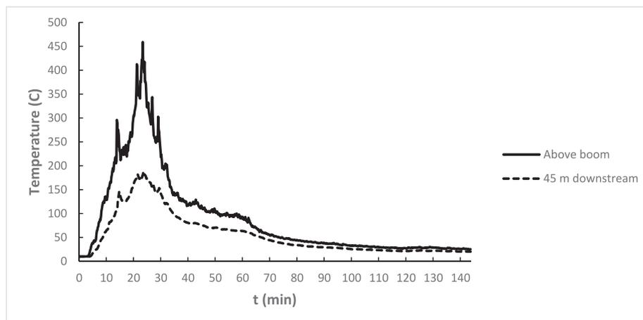
Fig. 2. The fire gas temperature above the boom and 45 m downstream of the fire–fire experiment involving a drilling rig [19].
