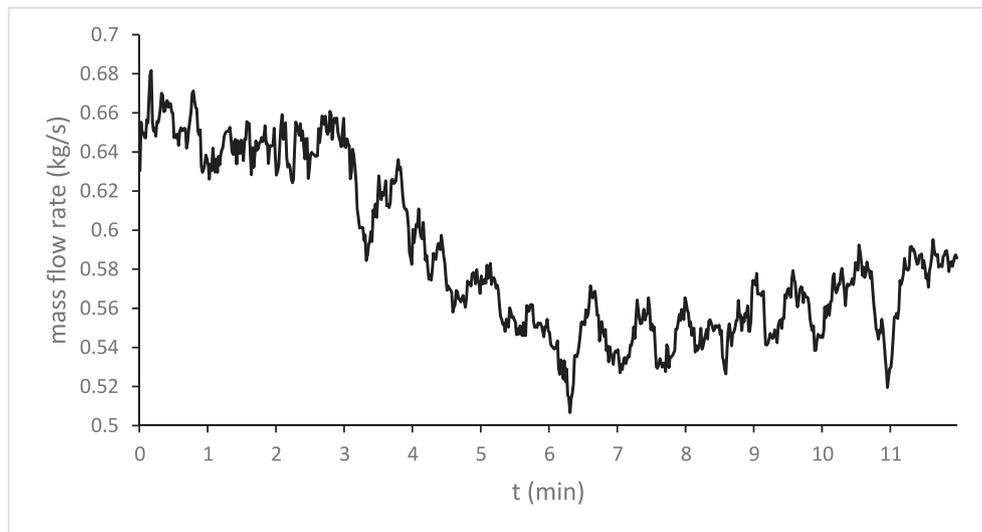
Fig. 4. The mass flow rate of a fire experiment in a model-scale mine drift, experiencing the throttle effect.
