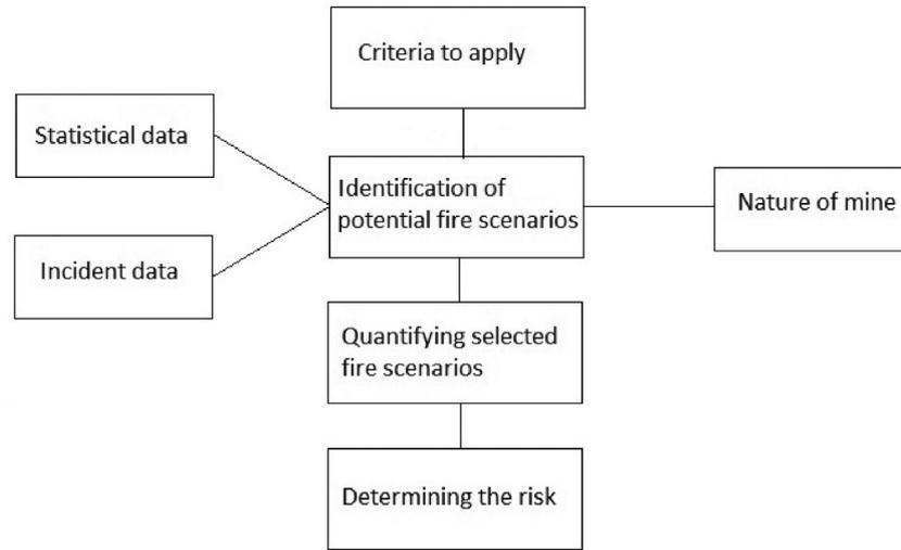
Fig. 1. The process of development and evaluation of design fire scenarios.
