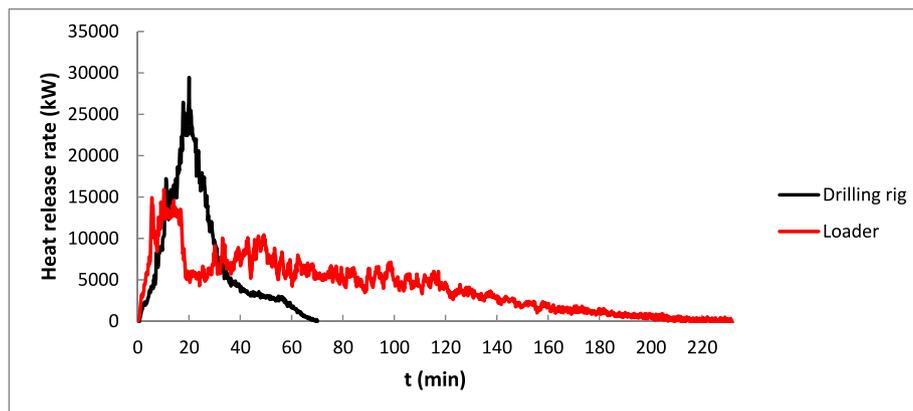
Fig. 3. The heat release rates of the full-scale fire experiments involving a loader and a drilling rig, respectively [19].
