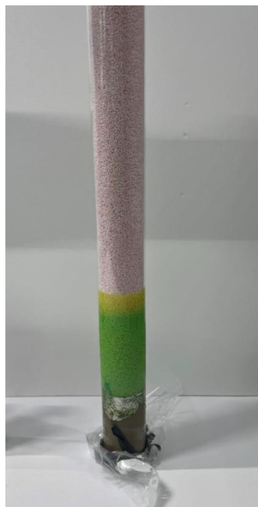
Fig. 3. ANFO samples in a graduated cylinder (equivalent to 9.0% humidity).
