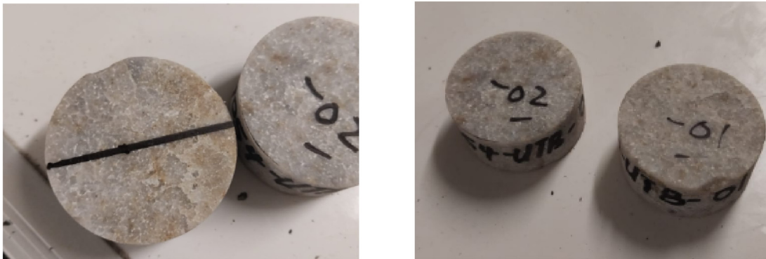
Fig. 8. Specimen prepared for indirect tensile strength (Brazilian test).
